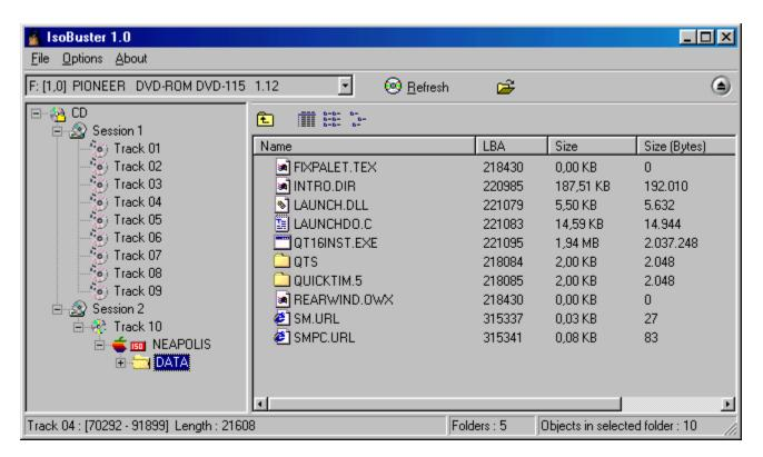
Another variant used to combine Audio with Data is the so called <u>Mixed Mode CDs</u>. They contain both audio and data tracks in the first session. The first track is a data track (where the Operating system will look for File System) the remaining tracks are audio tracks. A standard audio player of today will skip the first data track and proceed with the audio tracks, older audio players could get into problems trying to play the data tracks (Hence the use of Enhanced CD).
