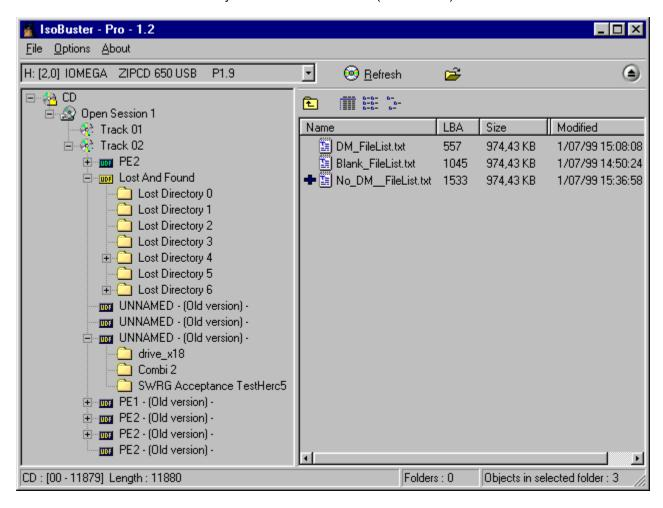
If IsoBuster detects errors during the scan, those sectors are marked. After the scan and **if** files are affected by errors (e.g. the files are located in erronous sectors) IsoBuster generates a list of all files that are affected. You can edit, save, print, ... this list.
