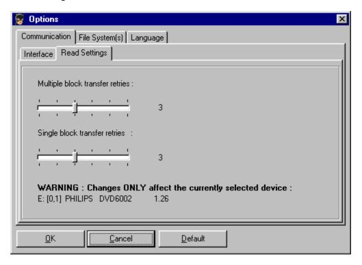
During reading, IsoBuster will typically (and where possible) read more than one block at a time. If that fails for some reason IsoBuster will read every block individually.
