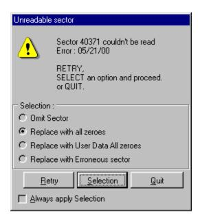
This Error Message can occur when you're extracting data (from CD, DVD or image file) to an image file, raw. It offers you to RETRY reading the sector, apply an option from the SELECTION window or to QUIT. The possible selections are :
