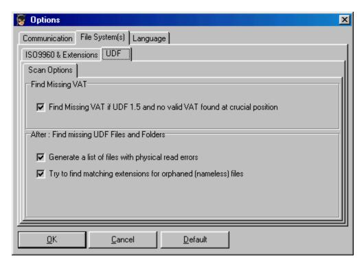
IsoBuster interprets UDF based on the UDF rules but while doing so also already looks further to see if it can't compensate for errors. One extra feature which is default set **on** can be switched off. This feature automatically looks for the last valid VAT.
